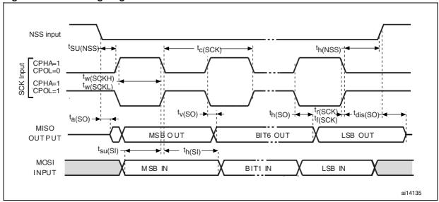
1. Measurement points are done at CMOS levels:  $0.3V_{\rm DD}$  and  $0.7V_{\rm DD}$ .
