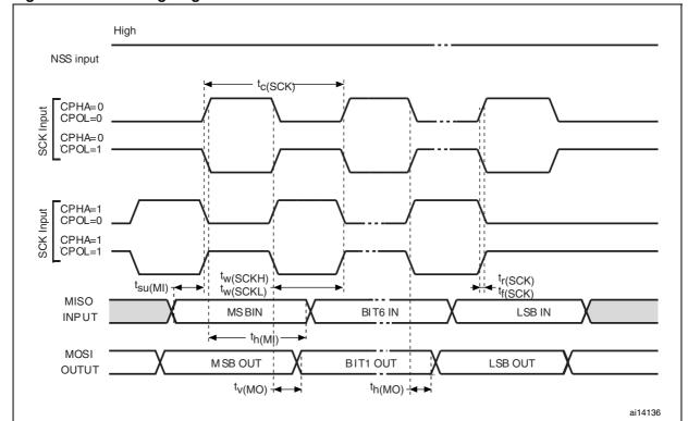
Figure 31. SPI timing diagram - master mode<sup>(1)</sup>
