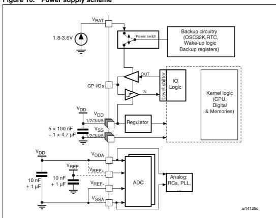
Caution: In Figure 10, the 4.7  $\mu$ F capacitor must be connected to  $V_{DD3}$ .
