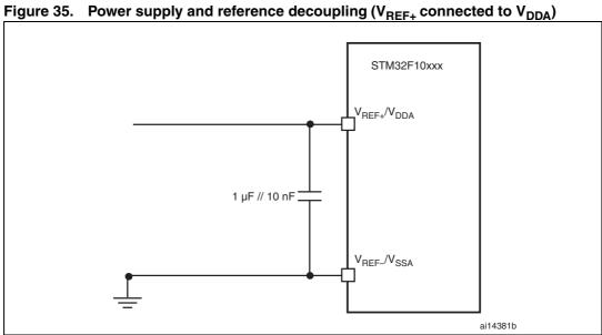
V<sub>REF+</sub> and V<sub>REF-</sub> inputs are available only on 100-pin packages.
