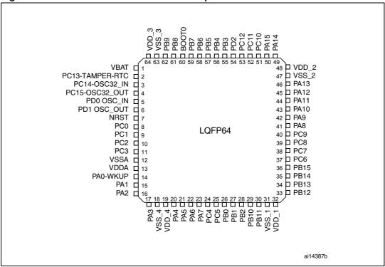
Figure 4. STM32F100xx value line LQFP64 pinout
