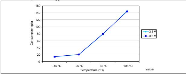
Figure 16. Typical current consumption in Stop mode with regulator in Low-power mode versus temperature at  $V_{DD}$  = 3.3 V and 3.6 V
