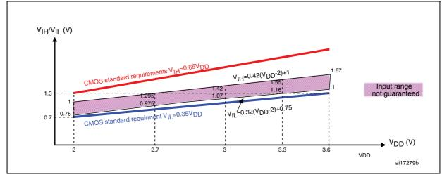
Figure 24. 5 V tolerant I/O input characteristics - CMOS port
