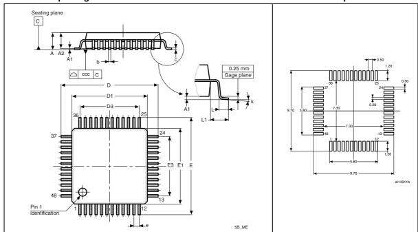
Figure 43. LQFP48 – 7 x 7 mm, 48-pin low-profile quad flat Figure 44. Recommended package outline<sup>(1)</sup> footprint<sup>(1)(2)</sup>
