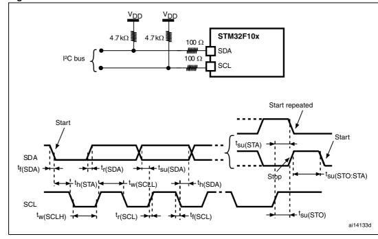
Figure 28. I<sup>2</sup>C bus AC waveforms and measurement circuit<sup>(1)</sup>
