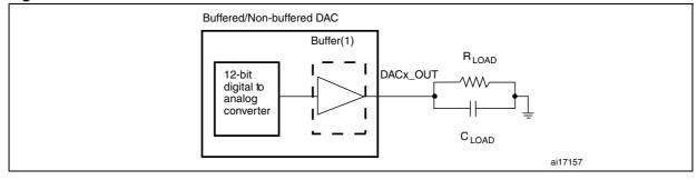
The DAC integrates an output buffer that can be used to reduce the output impedance and to drive external loads directly without the use of an external operational amplifier. The buffer can be bypassed by configuring the BOFFx bit in the DAC\_CR register.
