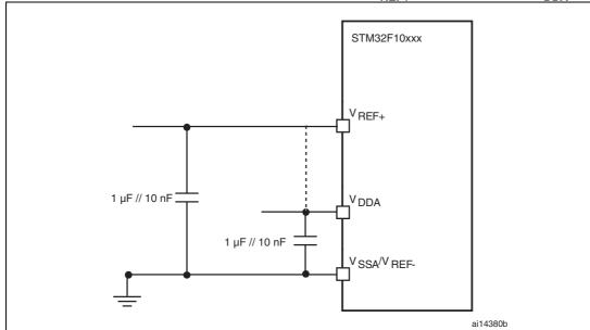
Figure 34. Power supply and reference decoupling ( $V_{REF+}$  not connected to  $V_{DDA}$ )
