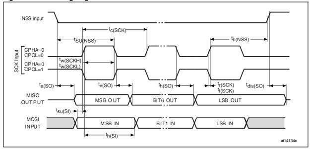
Figure 29. SPI timing diagram - slave mode and CPHA = 0
