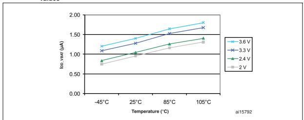
Figure 15. Typical current consumption in Stop mode with regulator in Run mode versus temperature at  $V_{DD}$  = 3.3 V and 3.6 V
