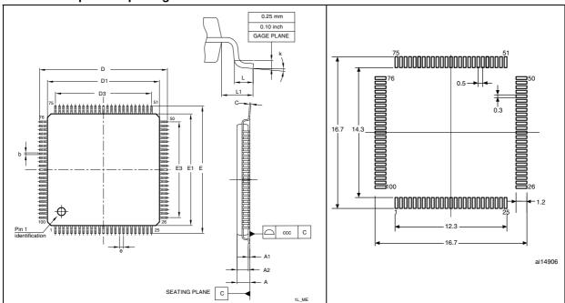
Figure 37. LQFP100, 14 x 14 mm, 100-pin low-profile Figure 38. Recommended footprint<sup>(1)(2)</sup> quad flat package outline<sup>(1)</sup>
