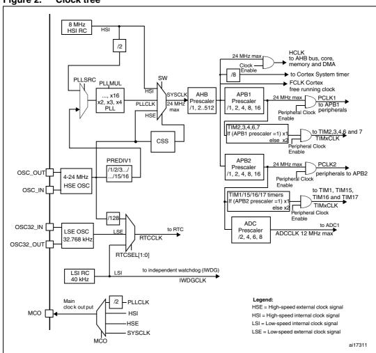
4. To have an ADC conversion time of 1.2  $\mu$ s, APB2 must be at 24 MHz.
