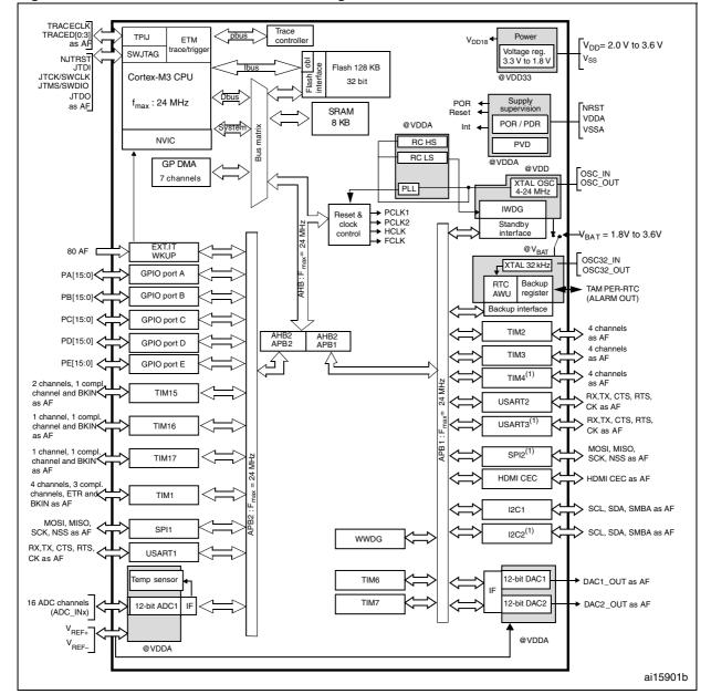
Figure 1. STM32F100xx value line block diagram
