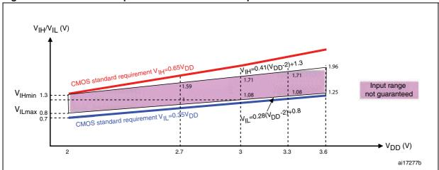
Figure 23. Standard I/O input characteristics - TTL port
